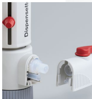
Valve system designed without seals
